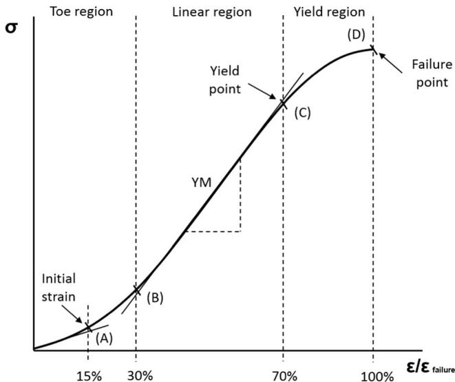
Fig. 3. Scheme of typical stress–strain curve for tendon tissue normalized to strain failure, identifying regions and proportionality ratios. YM - Young's modulus.
