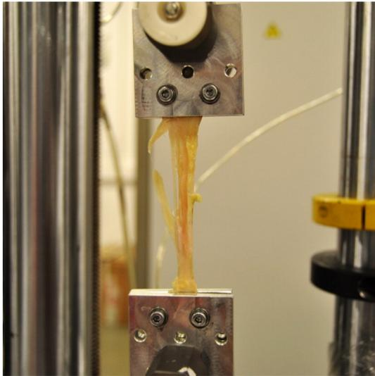
Fig. 2. Peroneus Brevis sample in the universal testing machine during test.
