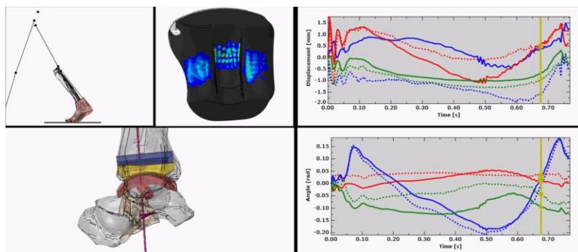
Figure 4 : Prosthesis insert contact pressure and joint ankle ROM during stance phase : with prosthesis (full lines) and without prosthesis (dotted lines).
