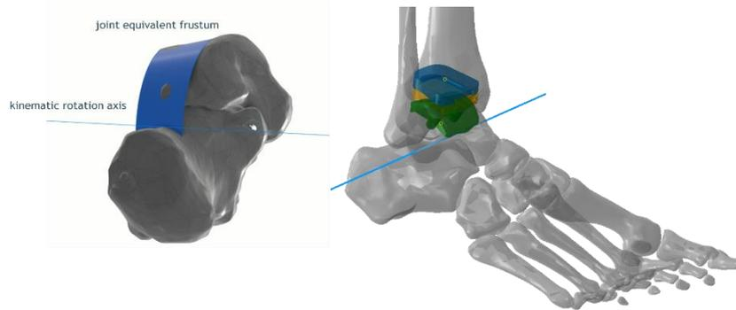
Figure 3 : Talus dôme equivalent axis of rotation (left); aligned reference prosthesis (right)
